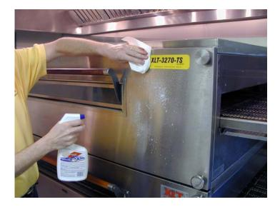
Clean front of oven with a soft cloth or rag and cleaner. Wipe in the direction of the grain
