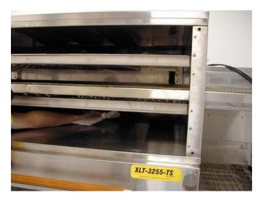
Wipe the interior chamber top, side walls, and floor as required to remove grease and other materials.
