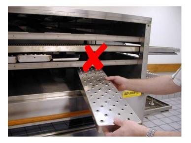
Due to the tapered shape, as well as buildup of material on the bottom of the oven, removal may be difficult with the finger cover in place.
