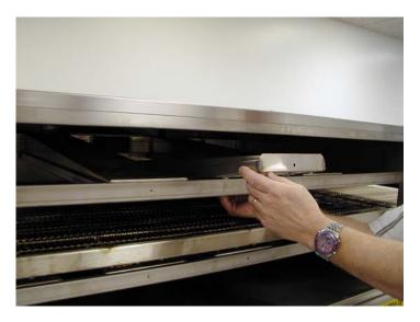
**Caution:** As soon as the finger is moved forward to clear the rear support it will drop to the conveyor unless supported.
