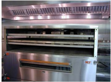
Once you have access to the interior of the oven, remove any large pieces of debris from the chamber floor.
