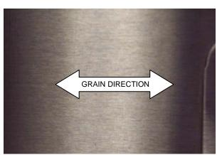
The exterior surface of your oven has a texture or "grain". When cleaning, follow the grain of the surface to help maintain the proper appearance.
