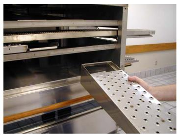
Continue this process for removal of the remaining fingers. Reverse the process to replace the fingers after cleaning.
