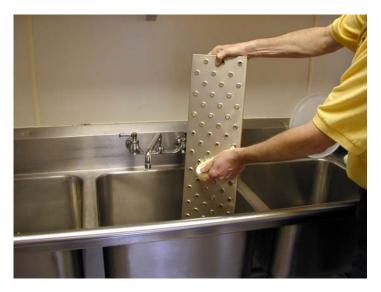
Lightly soiled finger covers may be cleaned by soap and water. A brush is recommended for use due to the raised openings.
