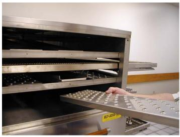
The finger body may remain in the oven after the cover has been removed. Repeat for all lower fingers.
