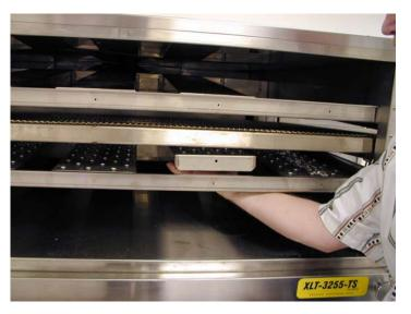
**Note:** Prior to removal of finger covers, please note location and configuration of covers for proper reinstallation.
