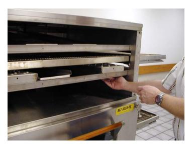
Lift the last finger clear of the front support. Pull it forward until it disengages the rear support.
