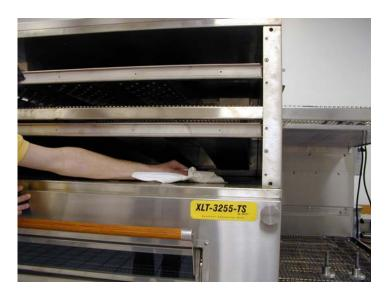
Remove the residue of any cleaning agents and wipe with a clean cloth.
