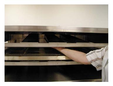
The upper fingers remove in a similar manner to the lower; lift the front end clear of the front support.
