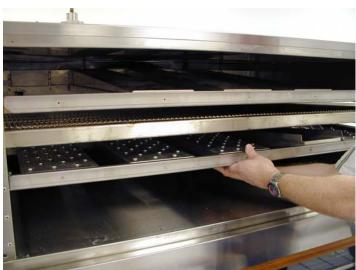
If the lower finger bodies need removal for cleaning (without removing the conveyor) follow this process:
