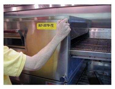
Remove the four (4) retaining knobs from the front panel.
