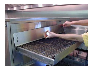
Remove the two (2) thumb screws and the conveyor flap.
