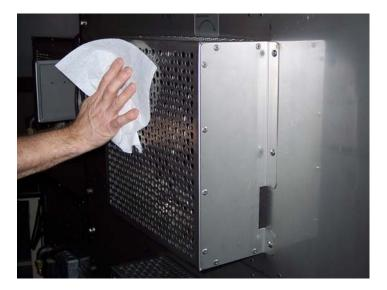
Clean top, back, and bottom of motor cover using a dampened cloth around breather holes. Do not spray cleaning agents into this area.
