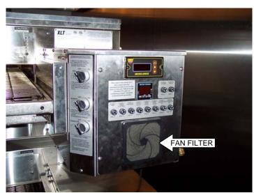
When cleaning the control box face and switches area, use a dampened cloth around controls, fuses, and switches. Do not spray cleaning agents in this area.
