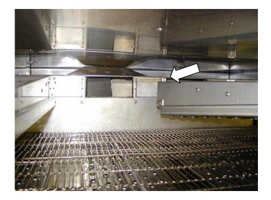
The upper fingers are slightly more difficult to position correctly. They nest against the back support smoothly (see arrow for incorrect alignment). Only replace fingers over open holes (some ovens have blocked holes). Refer to your notes or the finger chart included with the oven literature upon delivery.
