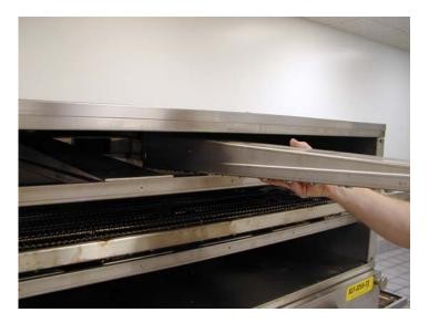
Lift the finger and pull it from the bake chamber.
