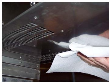
Clean underneath the control box using a dampened cloth around breather holes and labels. Do not spray cleaning agents into this area.
