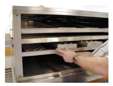
Pull forward until the back end of the finger body disengages from the rear support.
