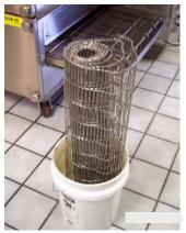
Once removed, the wire mesh belt may be washed or dipped as required to remove debris or grime. Caution should be used in all handling of the belt to avoid damaging the mesh.
