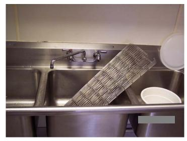
Rinse all cleaning agents from the mesh prior to reinstallation. Any abrasives left in the mesh can shorten the life of the belt.
