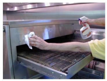
Remove accumulated grime from side of oven, control box, and conveyor cover. Repeat for the opposite side.
