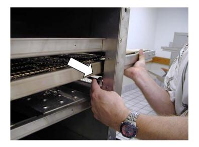
Place the knob (as shown) with the head against the face of the conveyor opening.
