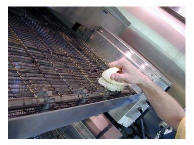
Typically, brushing the wire is sufficient for most belts.
