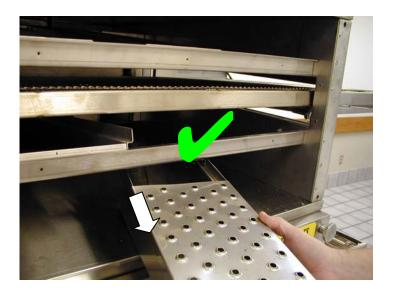
If additional clearance is needed, slide the finger cover forward a few inches to allow additional clearance.
