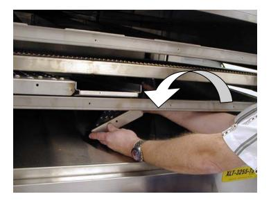
With a tilting/twisting action, rotate the unit left and down behind the front support bracket as shown.
